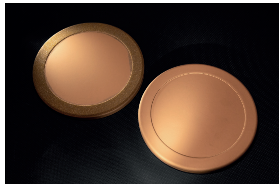
► Figure 3. SiC wafer carrier before (right) and after (left) several standard SiC epilayer processing runs.
